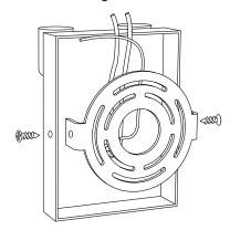
Attach the mounting bracket to the standard 4/0 electrical box using the two #8-32 screws provided. Make sure bracket is in level horizontal position.
