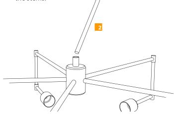
3 Slide the selected stems on the SVT/Clear wire cord down to the base of the fixture. The stems will screw into the base of the fixture and to each other to hide the threaded nipple.
