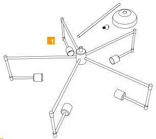
2 Figure out the length the fixture is wanted at with the stems.
