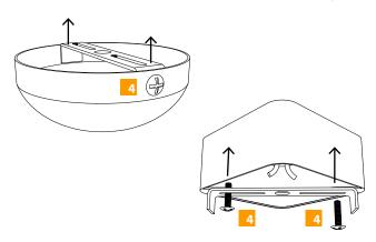
Once the stems are applied and screwed in take the canopy and ball joint and put them on the SVT/Clear wire cord. Canopy first followed by the ball joint. Slide down to the top of the stems, screw in the ball joint. Be careful with the canopy as the stems will be easy to scratch before this is mounted, the canopy floats until mounted.
