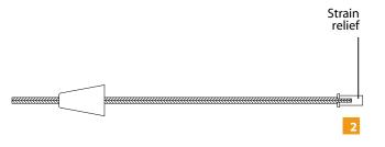
Insert the coaxial cable through the flared end of the strain relief.
