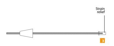
Insert the coaxial cable through the flared end of the strain relief.
