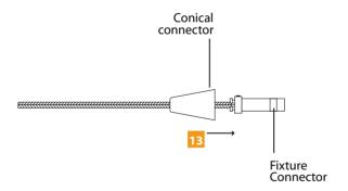
Slide the conical connector over the fixture connector.
