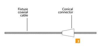
2 Insert the fixture coaxial cable through the conical connector
