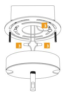
Connect 120V primary wiring (hot, neutral and earth ground) to the transformer input wires (black, white and green wires). Make sure connections are tight. Push the transformer unit towards junction box and slide the cross bar support screws through the transformer housing.
