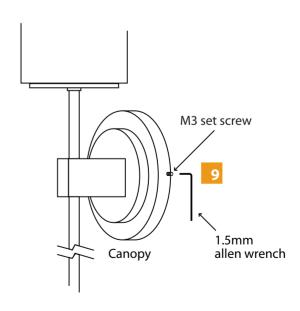
Place the fixture canopy onto the backplate. Level the fixture vertically and tighten the two M3 set screws with the 1.5mm allen wrench to secure the fixture in place.
