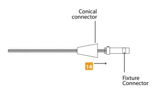
14 Slide the conical connector over the fixture connector.
