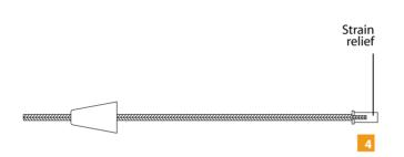
4 Insert the coaxial cable through the flared end of the strain relief.
