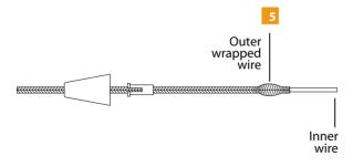
5 Slide the outer wrapped wire back to expose the inner wire.
